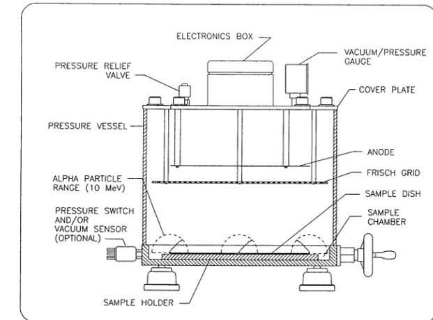
*Cut-away view of the Model 8210A Frisch-grid chamber*
